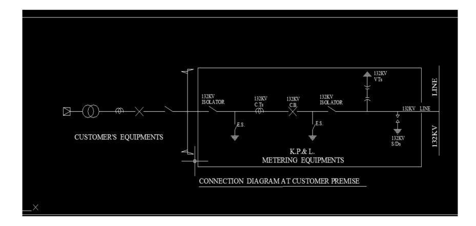
ii. General arrangement for BAMBURI 132kV METERING
